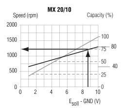
Minimum capacity setting 40% Maximum capacity setting 80% Measured voltage 8.7 V Speed is 1200 rpm
