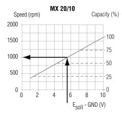
Measured voltage 5.5 V Speed is 1000 rpm
