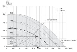
Speed 1200 rpm External resistance 120 Pa Air volume is 1900 m<sup>3</sup>/h
