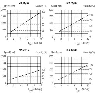
These graphs apply only if the minimum and maximum capacity setting has not been changed.
